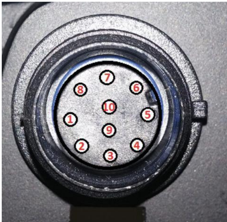
Figure. 3. GPIO pins as looking from the front face of the Spider
