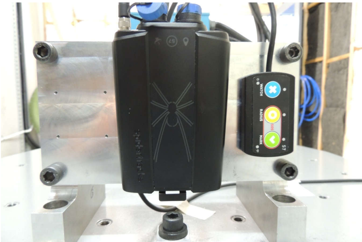
Figure 65: Vertical vibration pre test
