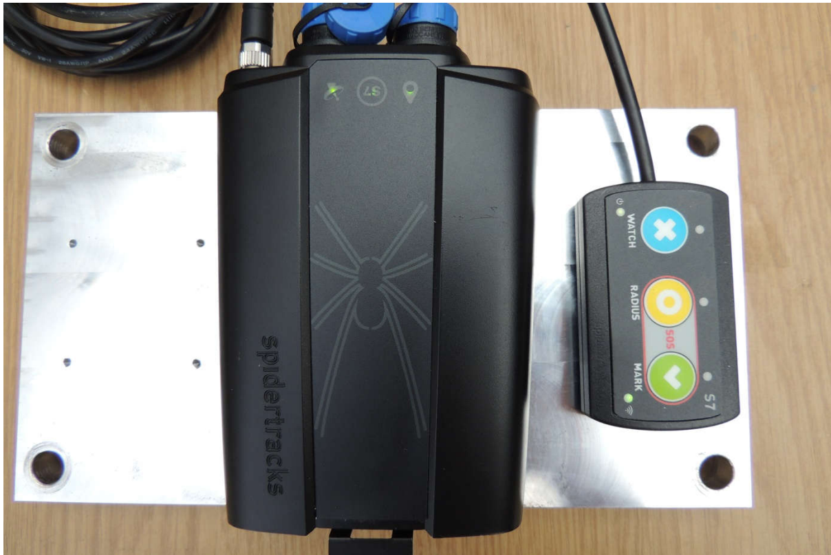
Figure 49: Fore vibration acceptance test
