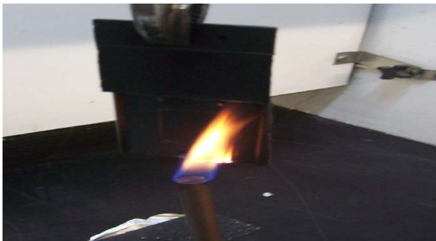
12 Second Flame Applied, Enclosure Bottom
