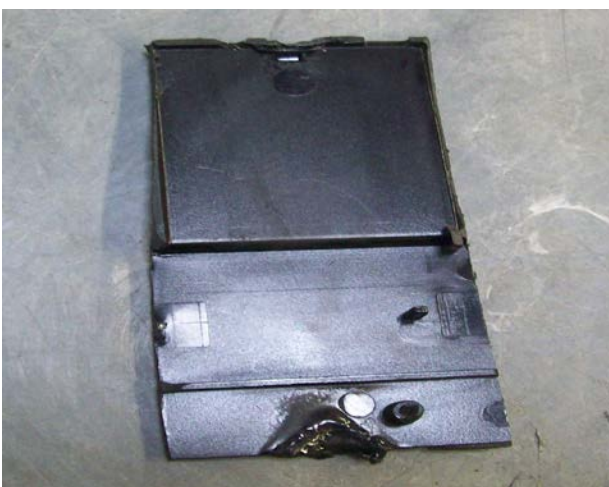
Burn Length, Enclosure Bottom
