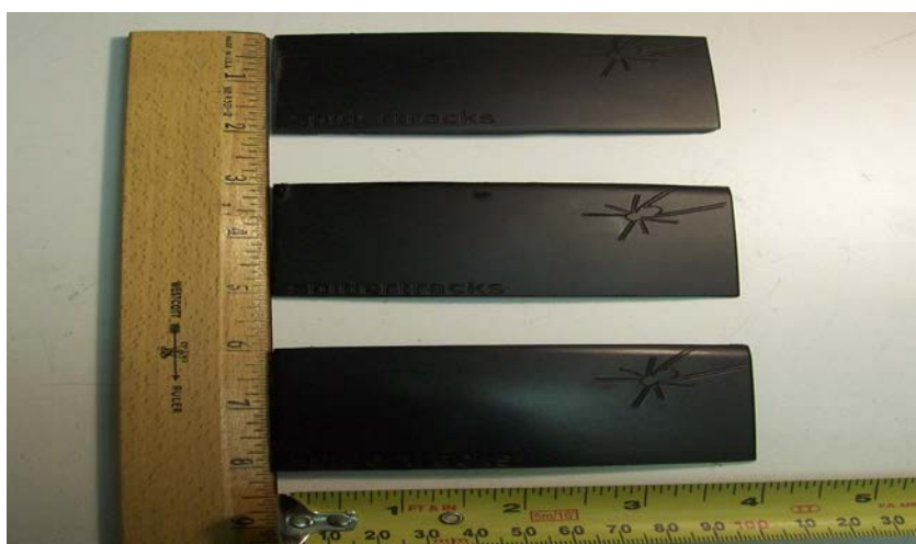
Test Specimens – Cut From S3 & S5 Enclosure Tops
