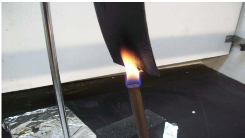
12 Second Flame Applied, Enclosure Top
