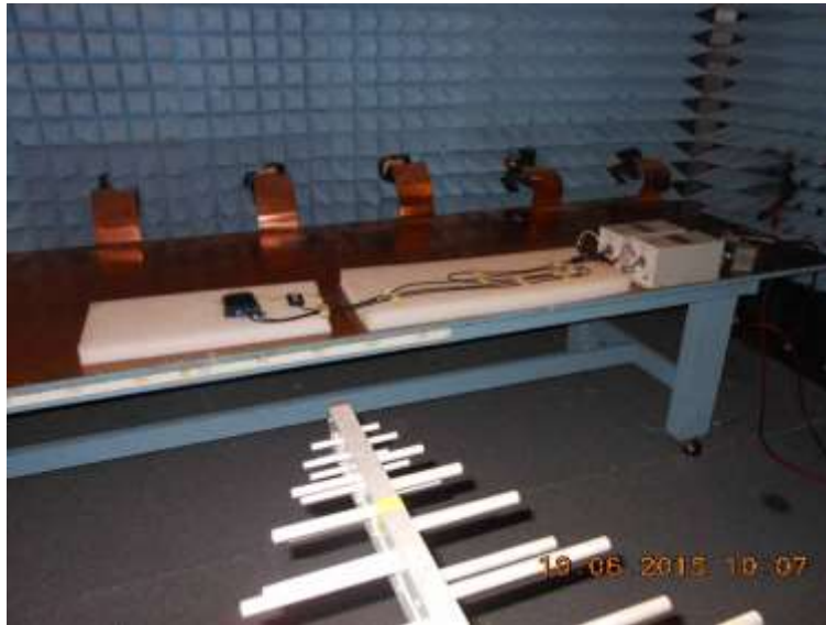
Section 21.5 - Log Antenna, 200MHz - 1GHz, Horizontal Polarization
