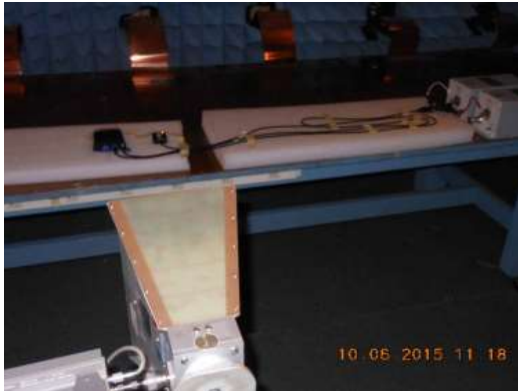
Section 21.5 - HF Horn Antenna, 1 - 6GHz, Horizontal Polarization
