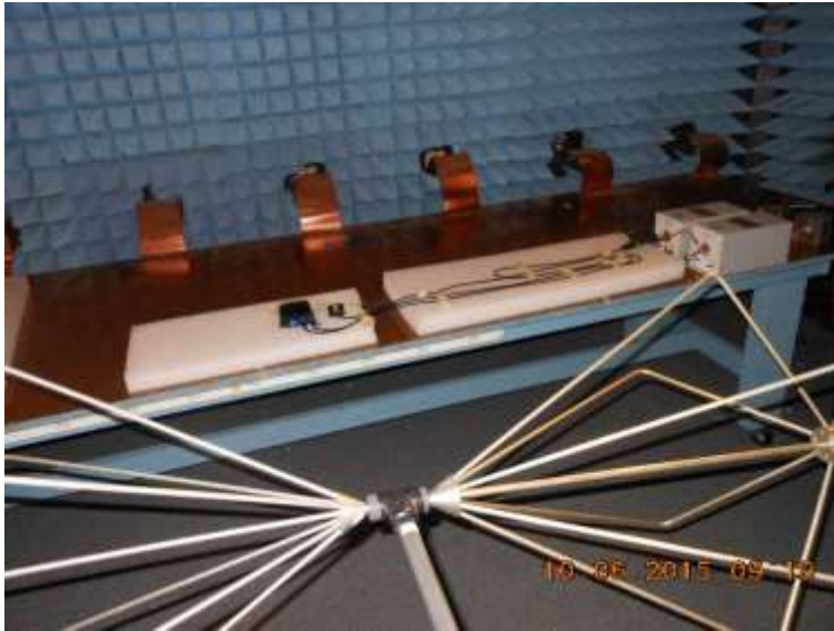
Section 21.5 - Bicon Antenna, 100 - 200MHz, Horizontal Polarization
