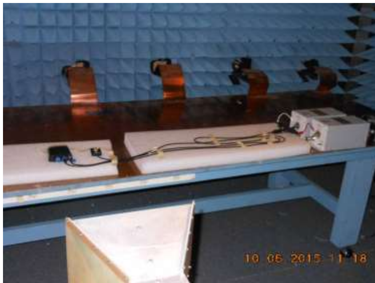
Section 21.5 - HF Horn Antenna, 1 - 6GHz, Vertical Polarization
