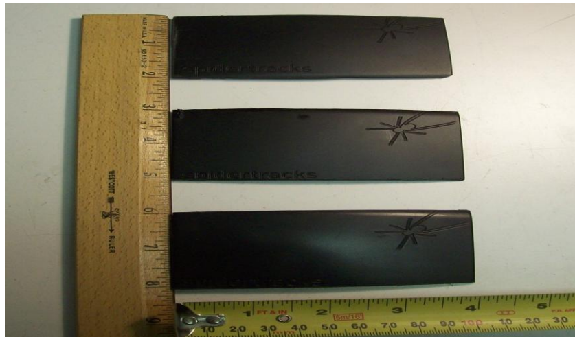
Test Specimens – Cut From S3 & S5 Enclosure Tops
