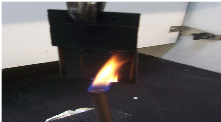
12 Second Flame Applied, Enclosure Bottom
