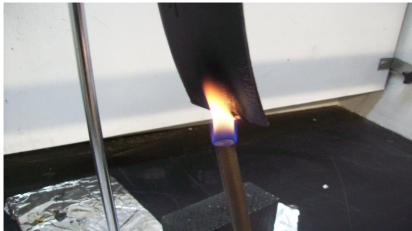
12 Second Flame Applied, Enclosure Top
