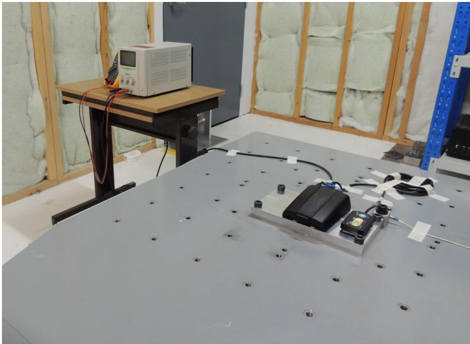
Figure 35: Vibration test setup
