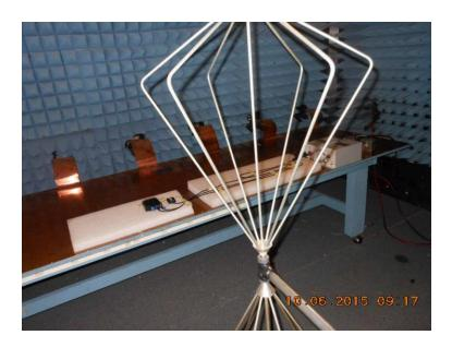
Section 21.5 - Bicon Antenna, 100 - 200MHz, Vertical Polarization
