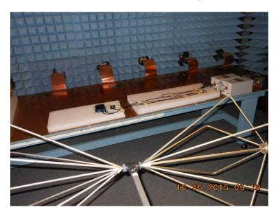
Section 21.5 - Bicon Antenna, 100 - 200MHz, Horizontal Polarization
