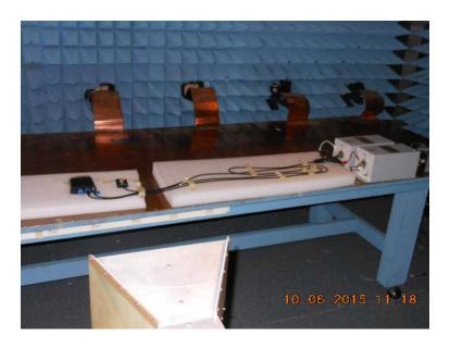
Section 21.5 - HF Horn Antenna, 1 - 6GHz, Vertical Polarization
