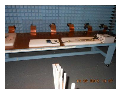
Section 21.5 - Log Antenna, 200MHz - 1GHz, Vertical Polarization
