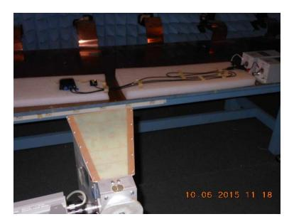
Section 21.5 - HF Horn Antenna, 1 - 6GHz, Horizontal Polarization
