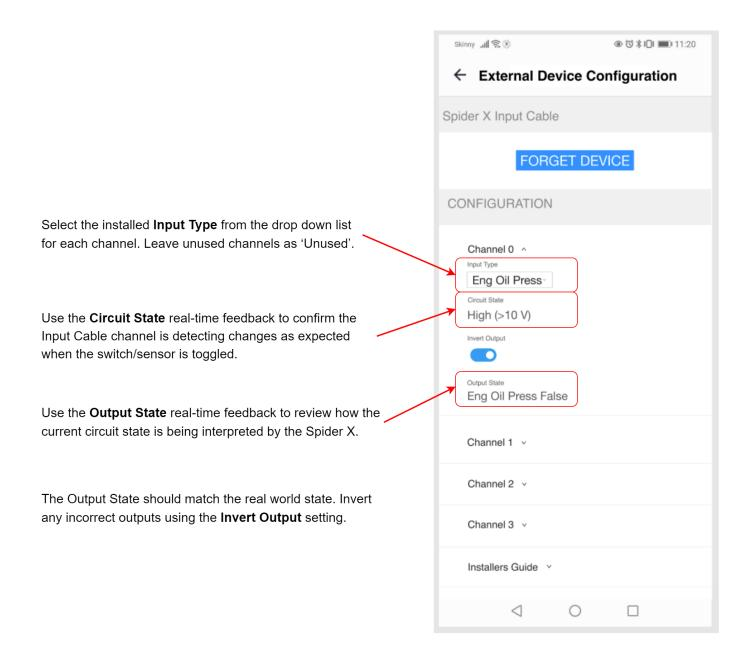
NOTE: Configuration changes are saved in real-time and stored in the Input Cable.
