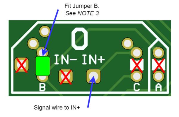
⚠ **NOTE 3:** When **Jumper B** is fitted, **signals must NOT be connected to IN-** of the same channel to avoid shorting signals to aircraft chassis/ground via the Spider X power supply.
