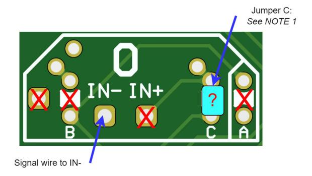
▲ **NOTE 1:** If the same switch is powering a load (e.g. indicator, instrument) then Jumper C should NOT be fitted. If there is no load, Jumper C should be fitted.
